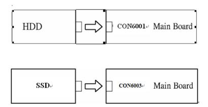
If any of the connections are loose, reconnect firmly and repeat Procedure 1. If there is still an error, go to Check 2.
